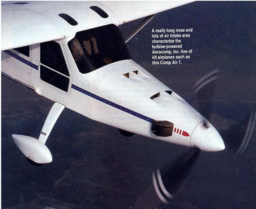
A really long nose and lots of air intake area characterize the turbine-powered AeroComp, Inc. line of kit airplanes such as this Comp Air 7.
